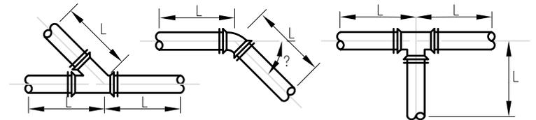
8. IF A CASING PIPE FALLS WITHIN THE RESTRAINED LENGTH "L", THIS REQUIRED RESTRAINED LENGTH "L" SHALL BE INCREASED BY THE LENGTH OF THE CASING.
