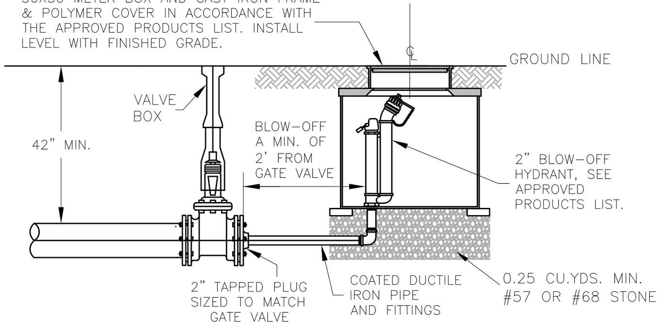
36X30 METER BOX AND CAST IRON FRAME & POLYMER COVER IN ACCORDANCE WITH THE APPROVED PRODUCTS LIST. INSTALL LEVEL WITH FINISHED GRADE.
