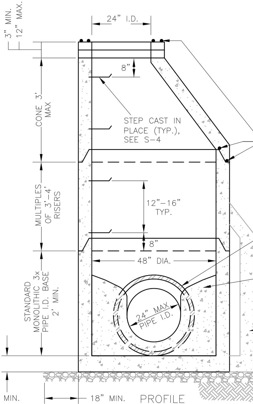
SEAL UNDER FRAME AND ALL JOINTS WITH 2 RINGS OF BUTYL RUBBER ROPE OR O-RING SEALER. ALL EXTERIOR JOINTS SHALL BE WRAPPED WITH A 6" (MIN.) WIDE WRAP IN ACCORDANCE WITH APPROVED PRODUCTS LIST AND MANUFACTURER'S REQUIREMENTS
