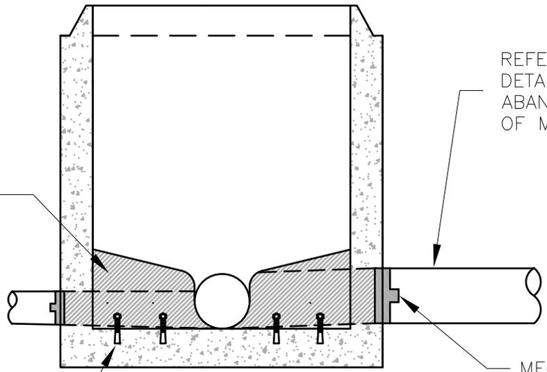
FILL ABANDONED INVERTS WITH 3000 PSI CONCRETE. MATCH EXISTING BENCH AND TROUGH GRADES.
