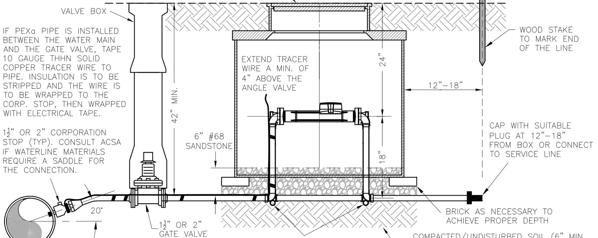
IF PEX<sub>d</sub> PIPE IS INSTALLED BETWEEN THE WATER MAIN AND THE GATE VALVE, TAPE 10 GAUGE THHN SOLID COPPER TRACER WIRE TO PIPE. INSULATION IS TO BE STRIPPED AND THE WIRE IS TO BE WRAPPED TO THE CORP. STOP, THEN WRAPPED WITH ELECTRICAL TAPE.
