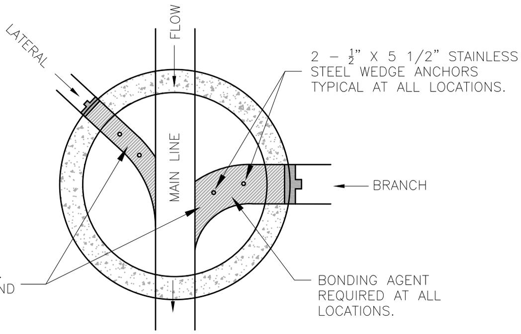
FILL ABANDONED INVERTS WITH 3000 PSI CONCRETE. MATCH EXISTING BENCH AND TROUGH GRADES.
