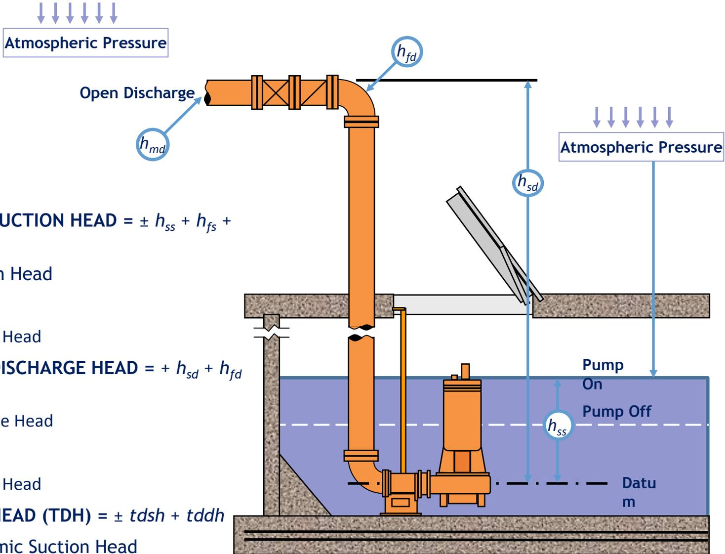
**TOTAL DYNAMIC SUCTION HEAD =  $\pm h_{ss} + h_{fs} + h_{ms}$**
