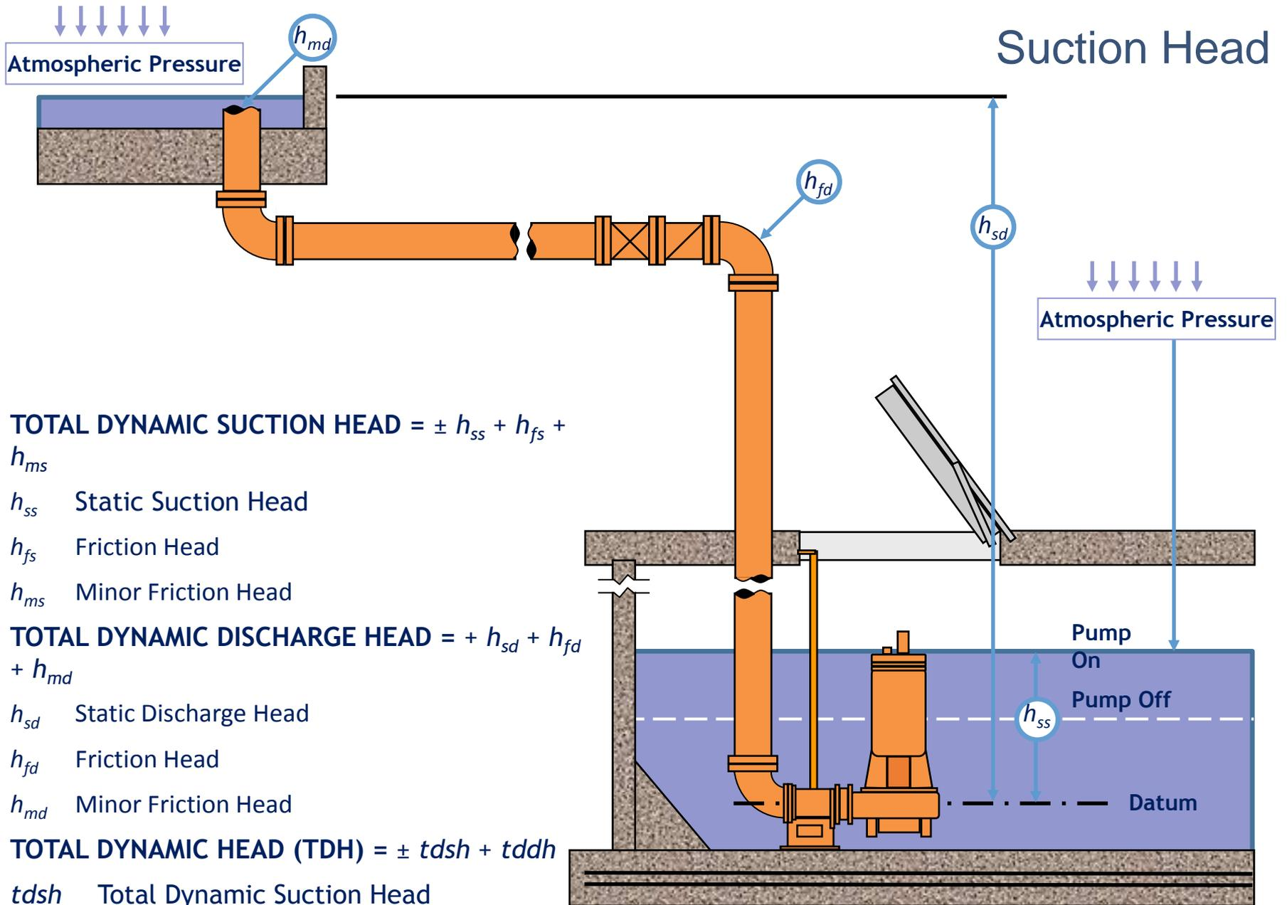
**TOTAL DYNAMIC SUCTION HEAD =  $\pm h_{ss} + h_{fs} + h_{ms}$**
