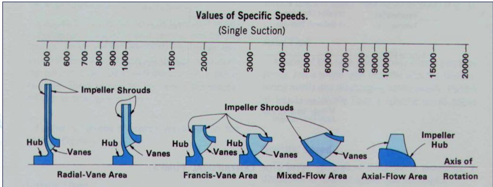
Fig. 5 Comparison of Pump Profiles
