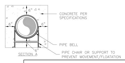
NOTES: ALL JOINTS IN ENCASEMENT SHALL BE MECHANICALLY RESTRAINED
